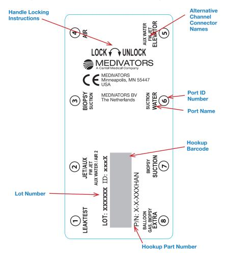
**Handle Locking Instructions** - insert block onto basin channel manifold and move handle to the left to lock. Move to the right to unlock.
