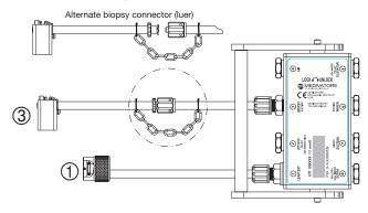
Each Advantage Hookup is comprised of multiple ports and connector assemblies. Each port is labeled with a Port ID number (circled). This same number also identifies the corresponding Connector Assembly. Each Connector Assembly is fitted with a specific endoscope connector. (see Fig. 2).
