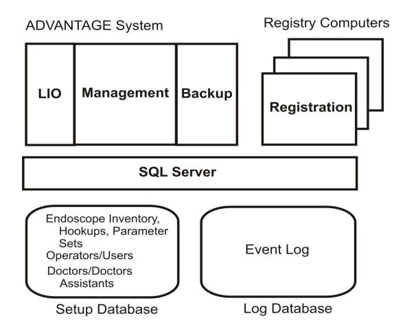
The ADVANTAGE System software is built upon the Windows XP platform. All features of Windows XP are available including an SQL Server. This platform allows configuring the ADVANTAGE System to support centralized administration.
