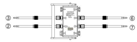
Each Advantage Hookup is comprised of multiple ports and connector assemblies. Each port is labeled with a Port ID number (circled). This same number also identifies the corresponding Connector Assembly. Each Connector Assembly is fitted with a specific endoscope connector. (see Fig. 2).
